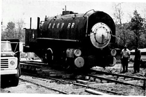
MAY, 1979: With tracks laid for loading, engine and wheels are placed on truck (above) at the locomotive's longtime resting place at Burnsville, N.C., in Yancey County. At right: Completing a route selected by the N.C. Department of Transportation to avoid low-hanging bridges, the dismantled locomotive arrives at Denton Airport.
